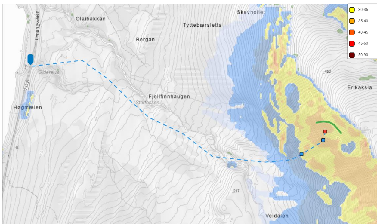
Figure 1 – Track and important points for the group the day of the accident. The blue marker is the starting point of the trip, the blue line is the route followed, the blue squares is the location of the snow pits dug, the red square is the release point, and the green line is the crown of the avalanche. The slope angle colour is found in the top right corner, and the blue areas are run-out-zones. All points and lines in this map are approximate positions and based on the memory and description of the event provided by the involved.
